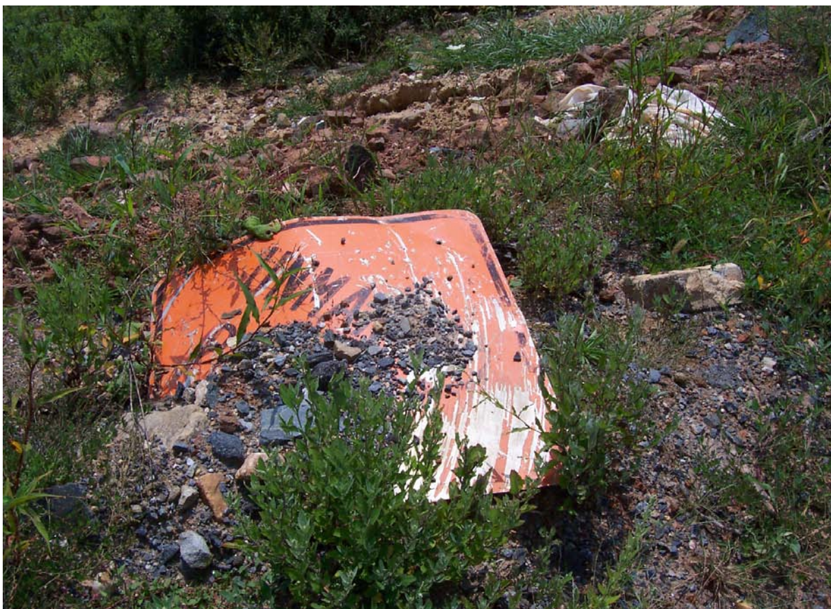
Above, August 29, 2007, Scarborough Landfill south side. Uncovered trash, erosion and spots of leachate.
